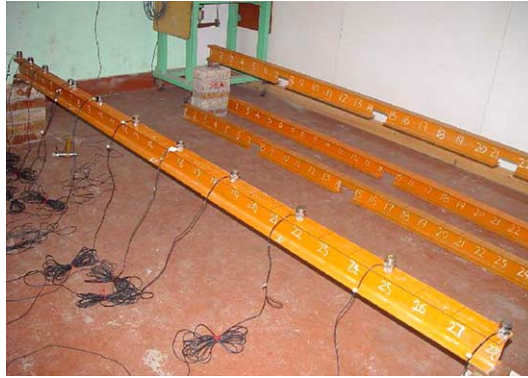
Fig. 9. Beam dynamic measurements in the laboratory.
